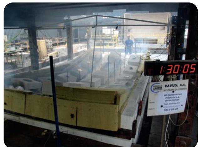
Fig. 12 Sample after 90 minutes – roof deformation protected with Isover FireProtect® is close to limit deformation given by test standard EN 1365-2 (fluent transition from bending stress to membrane)
