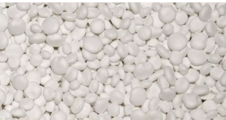
Fig. 13 – Raw material for the production of EPS
