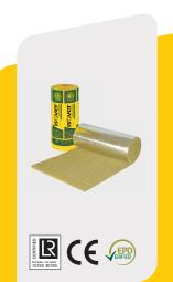
Specification code: MW - EN 14303 - T4 - ST(+)600 - WS1 - CL10
