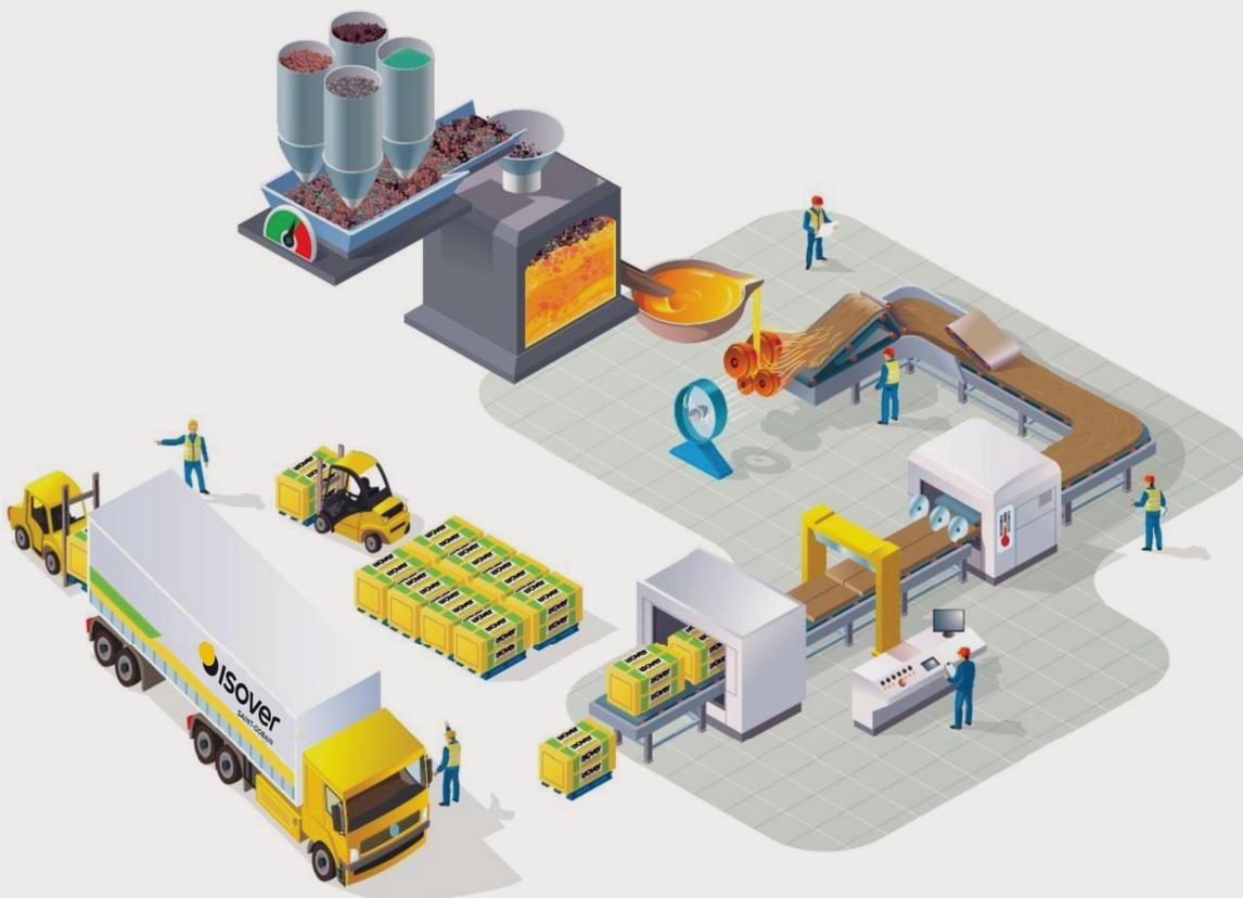
Fig. 3 - Manufacturing process schema
