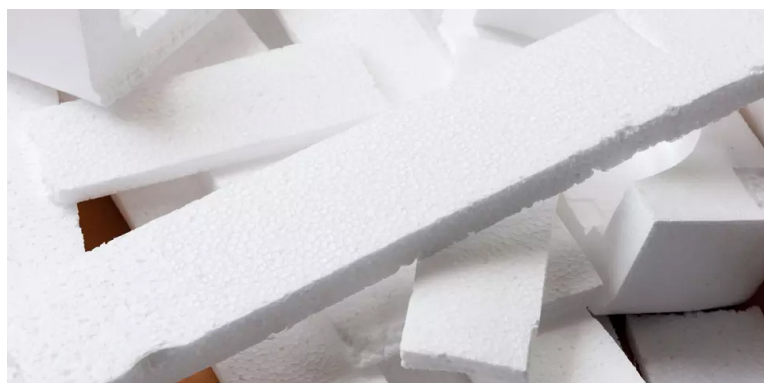
Fig. 14 - EPS offcuts from production
